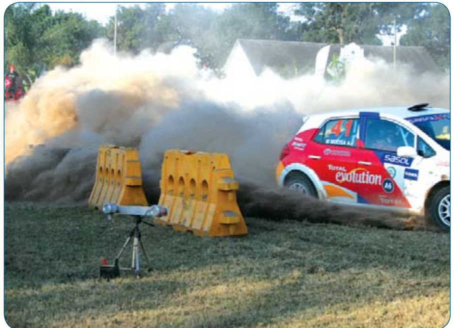
Fig. 1: Advances to the system include optional microwave barriers that can trigger at high speed in rain and dusty conditions.
