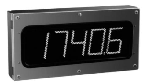
The Series 2000 are a range of extra large 3 to 5 digit LED array displays, 125 mm digit height, designed to be used in most process / temperature / weighing applications where high visibility and distant viewing is required. Using high intensity wide angle LED's in an IP65 enamelled steel housing ensures clear viewing distances of greater than 50 metres. For high ambient temperature conditions, an optional special coated glass window is available.
