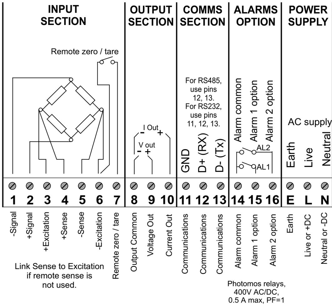
Interposing relays recommended for heavy duty applications
