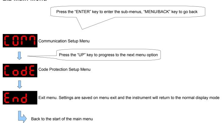
**Note:** The menu system has a 30 second program timeout. If no key has been pressed within this period then the instrument will save all settings and return to the normal display mode.
