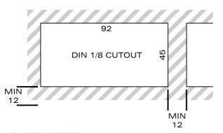
DIN 48  $\times$  96 industrial strength single piece housing Flame retardant ABS plastic, meets UL 94 V-0 rating Front panel IP65 (with o-ring seal supplied as standard)
