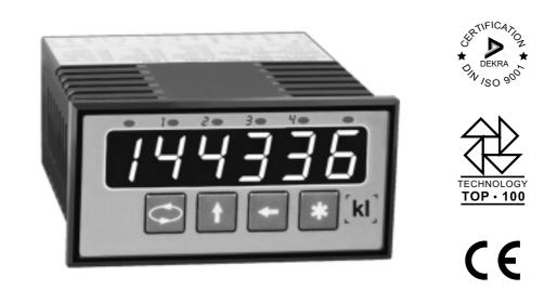
The Model 5012 is a 6 digit (-199999 to 999999) low-cost universal programmable indicator for use in all types of frequency & counting applications. The indicator has uni-polar & bi-polar pulse / frequency inputs for counting, frequency / speed (dual channel), period, flow, timing, totalising & positioning applications. It can be used in conjunction with most standard pulse / frequency generating sensors. Sensor excitation is standard & the output voltage is link selectable.
