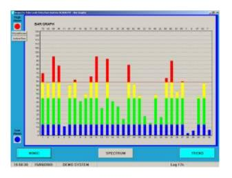
Bar graph mode has provision to display up to 32 processed sensor alarm signals simultaneously on the monitor. The vertical coordinate is the present alarm level and the horizontal is the sensor number. Under tube leak conditions, the graph climbs from the normal Green zone, to Yellow for caution, and to Red to show a critical situation has been reached. Fault Conditions and Low Sensor Levels are displayed in Blue.
