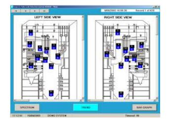
Mimic shows the boiler plant layout giving the position of each sensor. The vertical coordinate is the Boiler Level height in metres, and the horizontal is a pictorial display of the boiler layout. The sensor numbered points change colour on the monitor to indicate alarm conditions.
